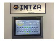
In our new generation of lubrication systems for presses all parameters of the spraying pattern can be controlled remotely controlled through a PLC. This is a necessary step toward full connectivity between machine parts and a central control station and therefore towards the so called Industry 4.0 or "internet of things".
